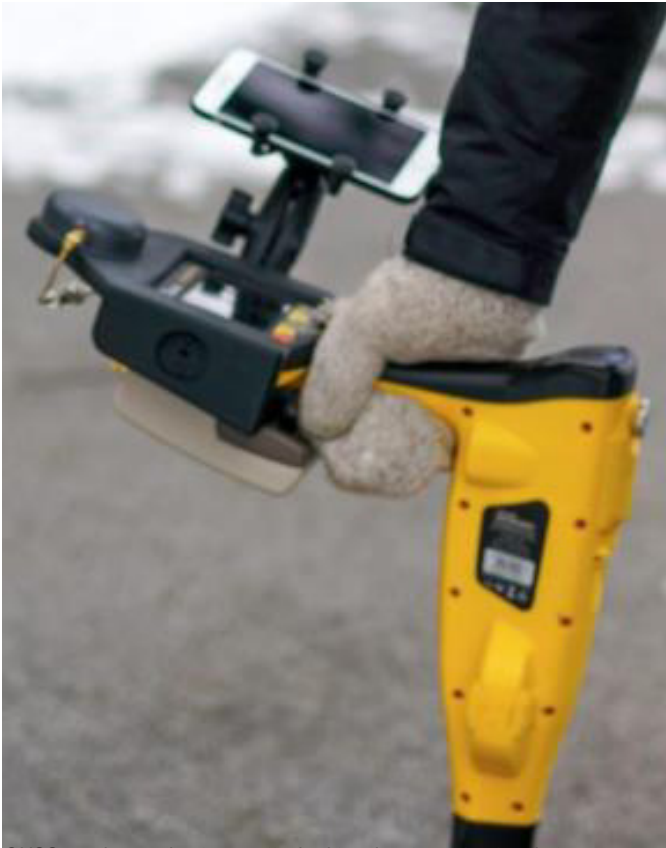
GNSS receiver and antenna attached to a locator with a bracket
