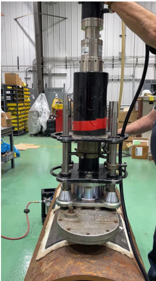
ALH System Three pneumatic Drilling and Tapping Machine installed on bonded saddle
