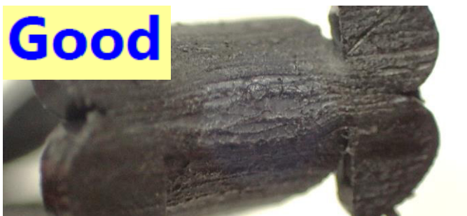
Examples of side-bend test results: ductile (left), non-ductile (right)
