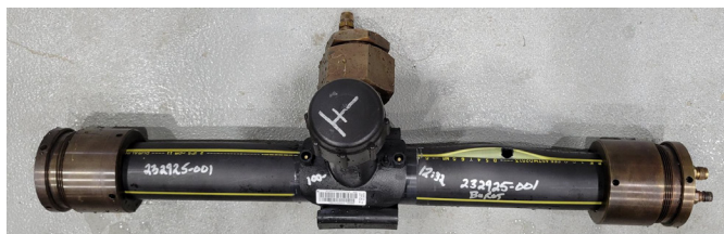
Test sample -post quick burst testing
