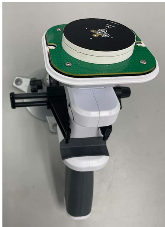
L-Band Mapper (cover removed)
