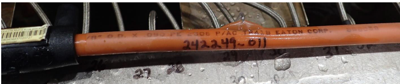
Specimen 242249-011, Ductile failure in pipe
