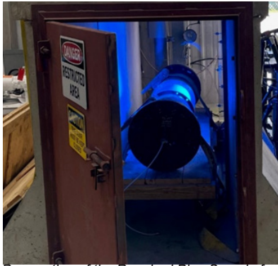
Preparation of the Repaired Pipe Sample for Internal Pressure Tests
