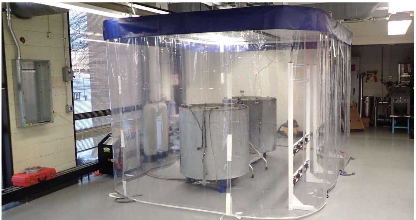
The enclosing test, water tanks, gas cylinder racks, water heaters, water-conditioning system, and ventilation duct are all in place.
