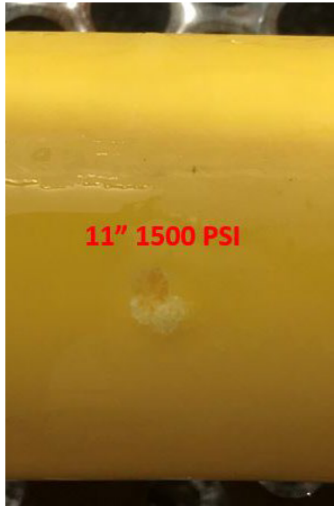
MDPE Pipe Punctured by 1500psi Straight Tip Water Nozzle at Height of 11in after 12sec
