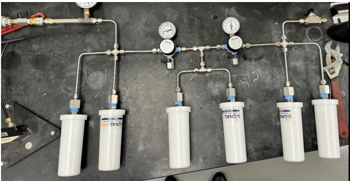
LoRaWAN-enabled Pressure Sensors Test Setup
