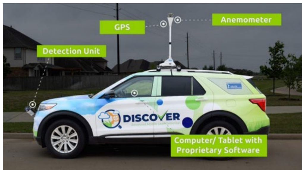
Discover AMLD system components (source: Discover Advanced Mobile Leak Detection- Product Brochure)
