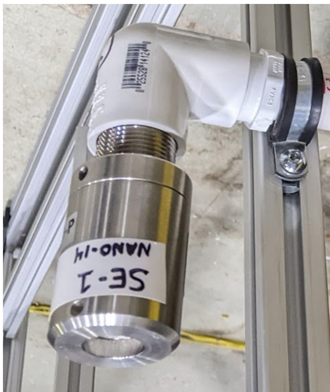
Methane sensor housing in a downward position.
