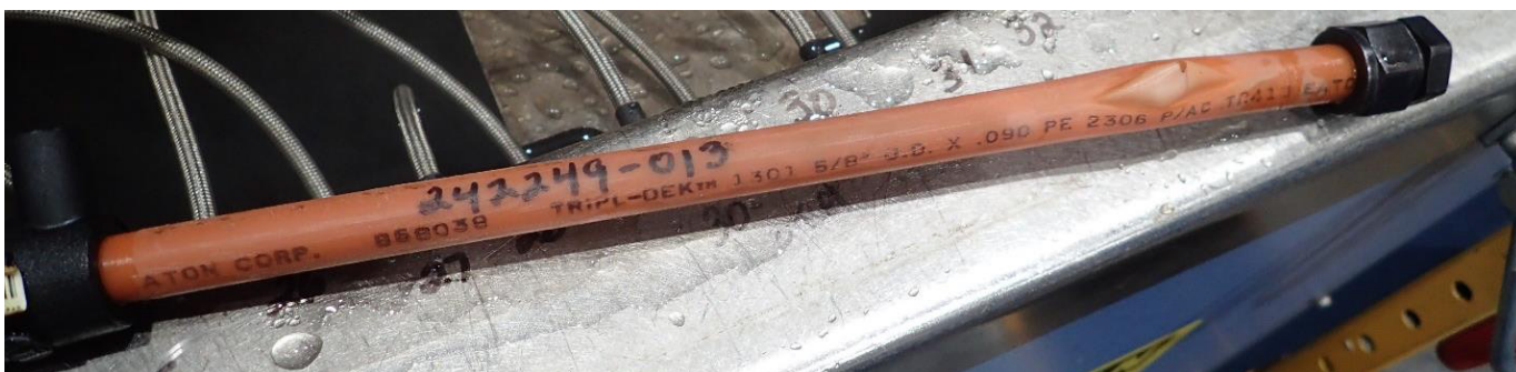
Specimen 242249-013, Ductile failure in pipe
