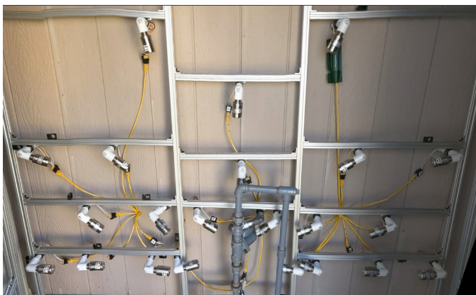
Methane sensor array with sensors positioned around the regulator vent.
