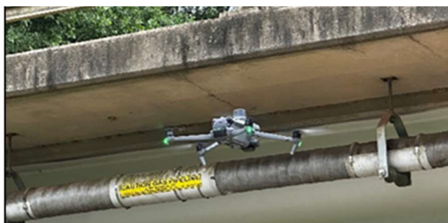
Left: A schematic showing the different “runs” or flight paths used by drone vendors to cover different angles and elevations of the pipe mounted under a bridge. Right: A photo of a drone surveying the pipe under the bridge. Figure credit: Left: Aerial Production Services, Right: Southern Cross.
