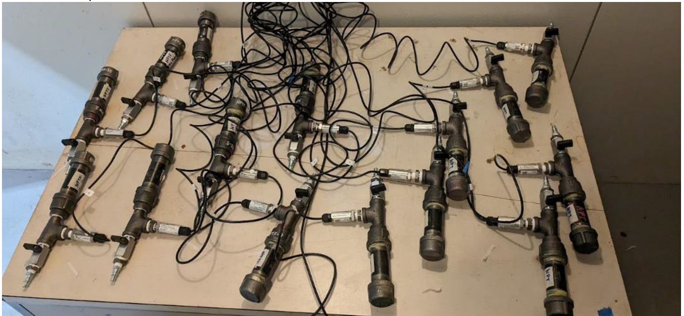
All samples are connected to pressure transducers inside the temperature chamber.
