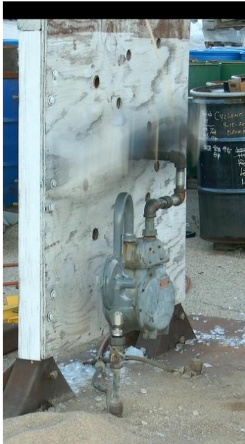
Figure 33: Falling 70 lb Sandbag Reinforced by Duct Tape – About to Impact Utility 1 Meter Set with Breakaway
