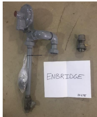
Figure 71: Utility 2 Meter Set
