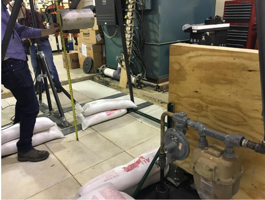
Figure 69: Tester Taking Measurement of Ram Release Height
