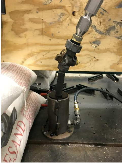
Figure 27: Utility 8 Retest – Sch 40 Riser – Impact Parallel to Wall from Regulator side – Street Valve Failure (Threads Into Street Valve Broke)
