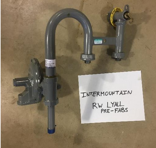
Figure 72: Utility 3 Meter Set
