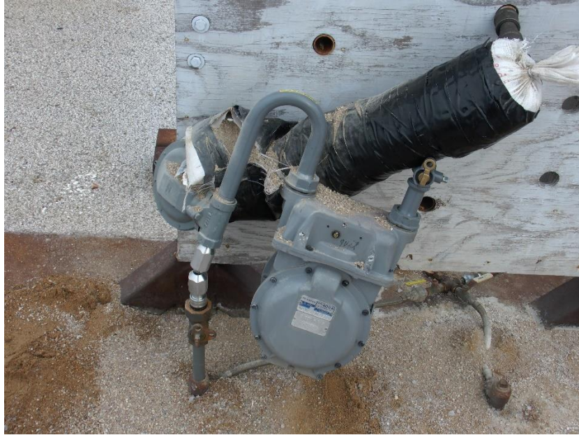
Figure 87: Questar Meter Set with Breakaway After Drop Test
