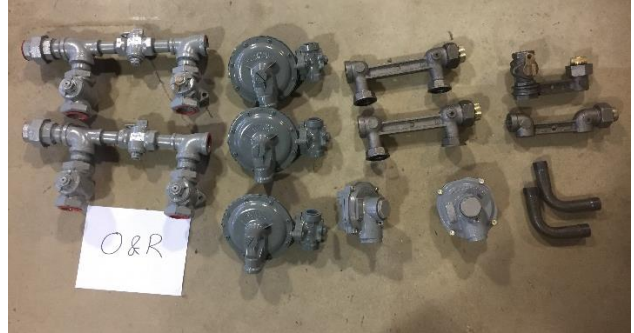
Figure 75: Utility 6 Meter Set Components
