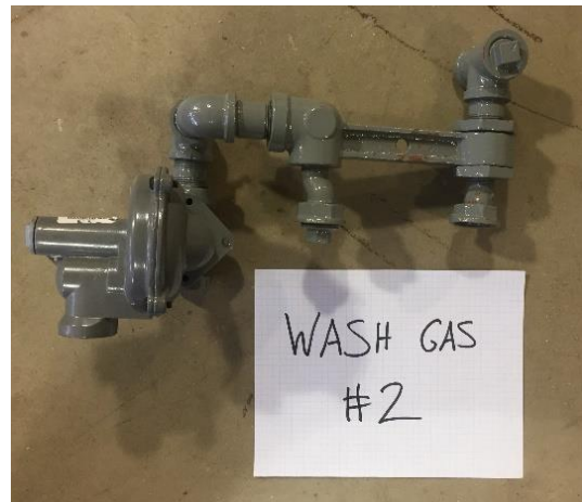
Figure 82: Utility 9 Meter Set #2 (Elbow Connections)
