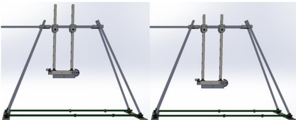
Figure 46: Adjustment of Height of Suspended Weight
