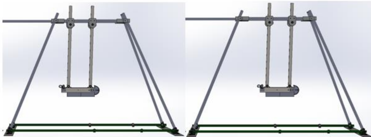
Figure 45: Movement of Custom Bushing Housings Along Horizontal Pipes of Frame
