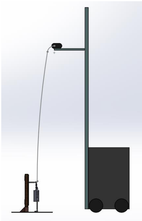
Figure 31: Side View of Path of Sandbag From Drop Test Setup
