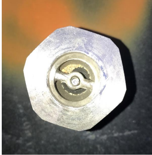
Figure 85: Bottom Half of Breakaway from Utility 1 Meter Set After First Drop Test – Sand Visible at Seal
