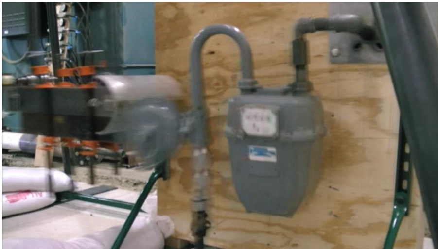
Figure 12: Impact Test on Utility 1 Meter Set with Breakaway and Regulator Left of Riser (Away from Meter) – Impacted Parallel to Wall from Regulator Side – After Impact
