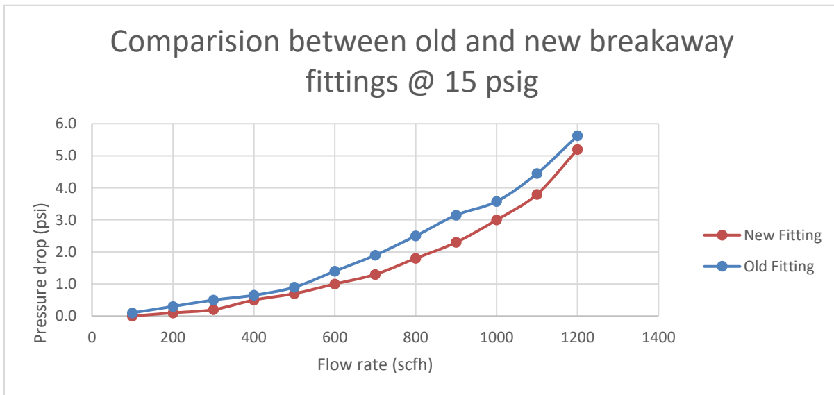
Figure 4: Comparison of Flow Testing Results Between Old and New Generation Breakaway Fittings at 15 psig
