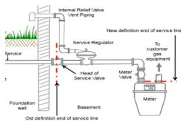
Researchers are developing best practices and guidelines for the retrofitting of inside gas service regulators and associated piping to maintain the same level of safety as a regulator installed outside. This project will provide the actions required to investigate, rehabilitate, and retrofit indoor gas regulators and piping systems.
