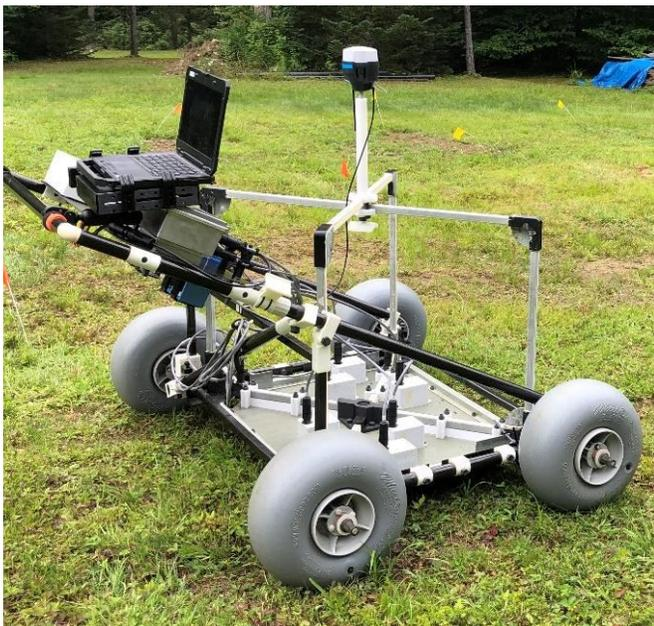
The solution is based on enhancing and adapting above-ground large-standoff 3D EM detection technology and supplementing the technology with an in-pipe mechanism to focus on congested areas and plastic materials. The combined solution will address most of the in-field conditions, including varying pipeline material, depth, and surface cover. The improved tools will provide access to the 3D data in near real time.
