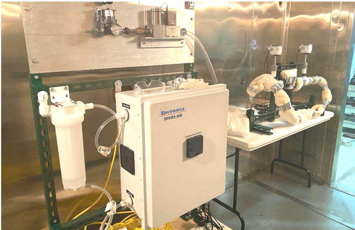
*Water-vapor removal test rig.*
