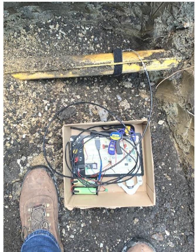
Field measurements on two-inch-diameter plastic main.
