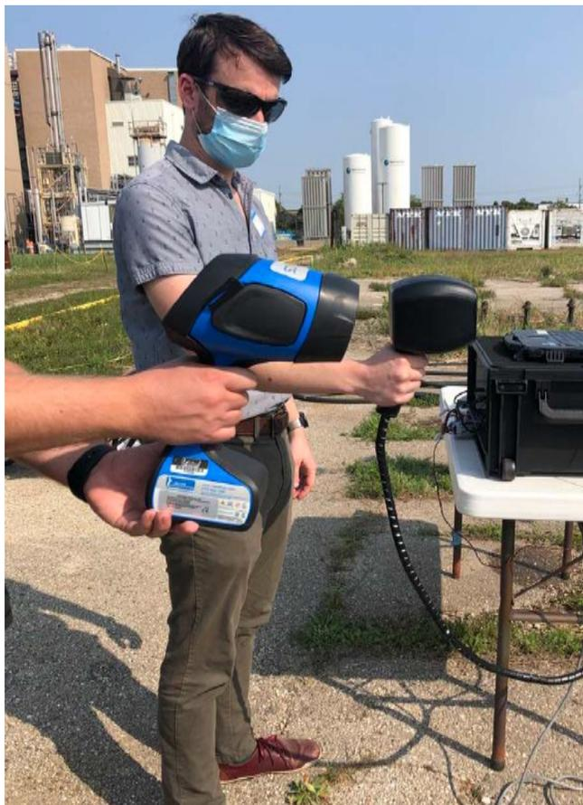
images of small fugitive leaks from municipal distribution pipelines and quantify the leak rates. The system was subsequently repackaged to be a portable, handheld unit.
