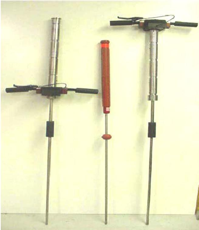
*Concept/prototype barhole tooling.*
