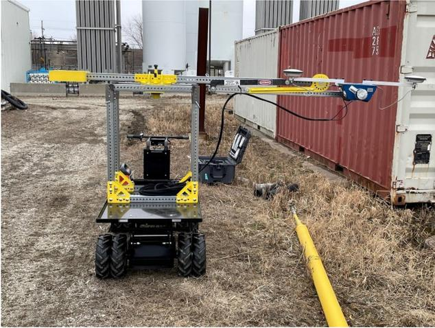
*Fully constructed pushcart with the scanner attached.*
