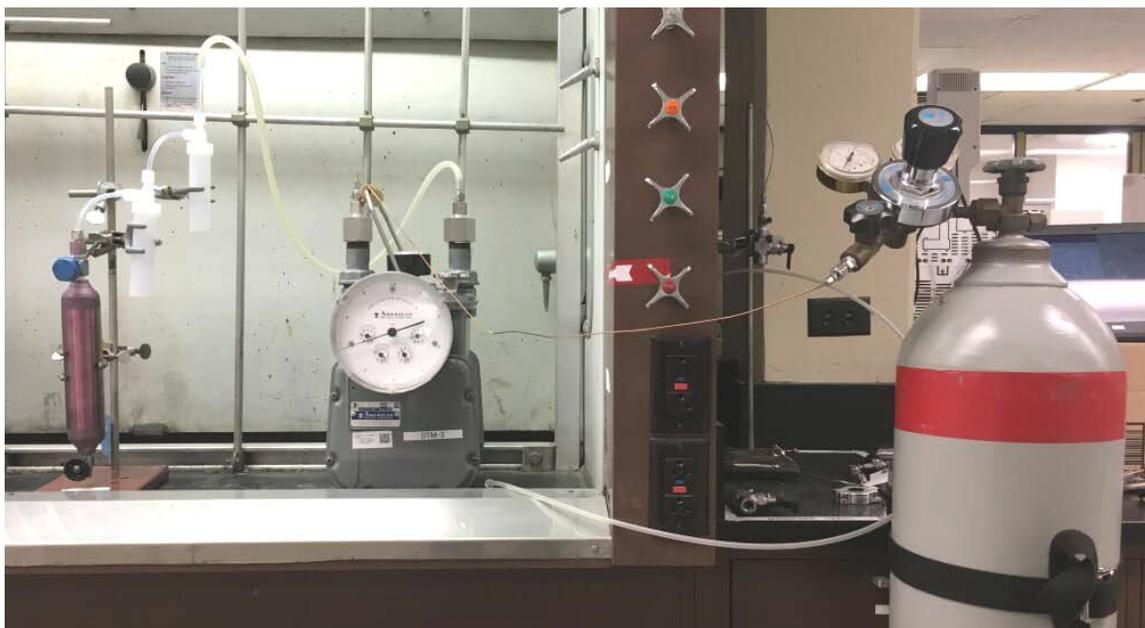
Setup to spike siloxane in methane gas.
