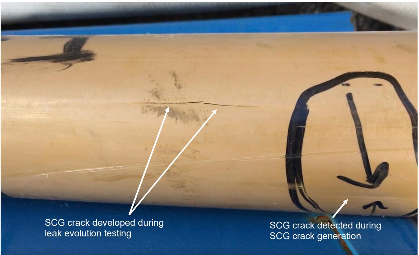
SCG crack developed during leak evolution testing
