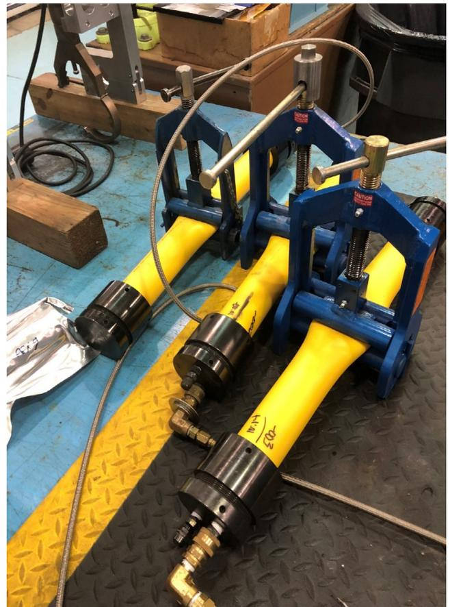
*Pipe samples squeezed-off under pressure.*
