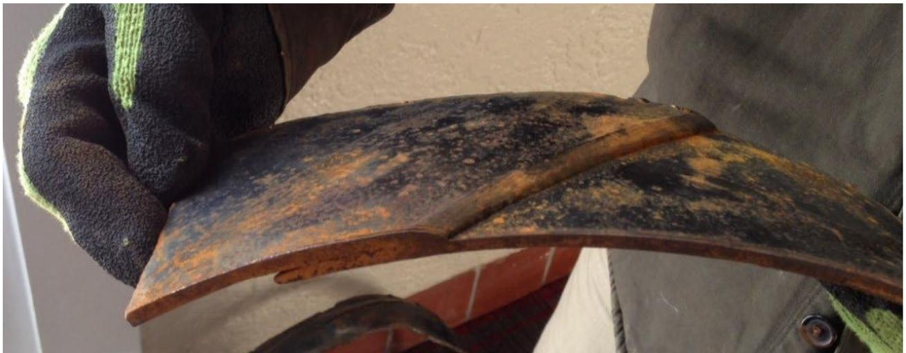
*Large-diameter lap seam spiral-welded pipe. (Image courtesy of K. Leewis.)*
