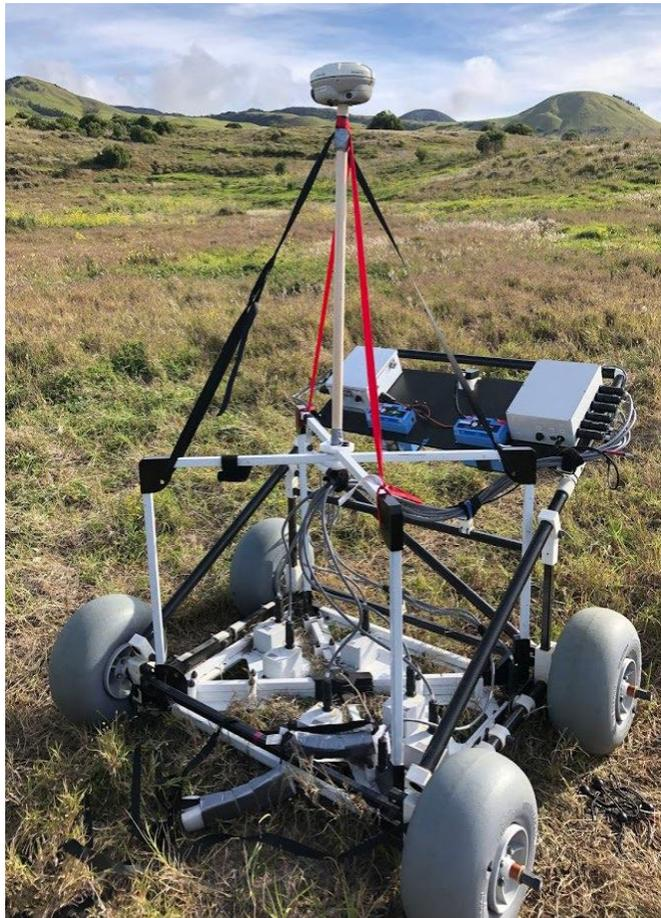
APEX is an advanced system for characterizing buried metal objects.
