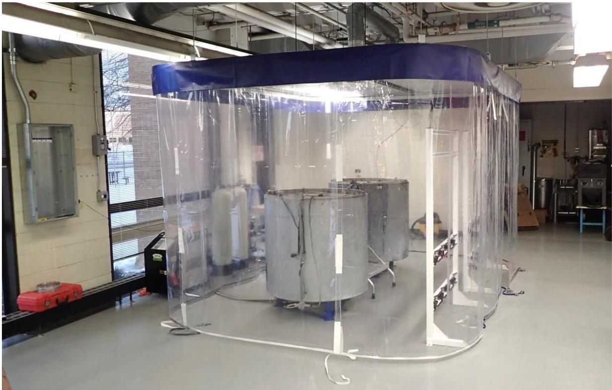
*The enclosing test, water tanks, gas cylinder racks, water heaters, water-conditioning system, and ventilation duct are all in place. The tent enclosure confines any gas release and ensures the gas will be quickly extracted through the vent duct at the ceiling of the enclosure.*
