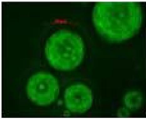
Smart corrosion-detector beads fluoresce a specific wavelength of light when in the presence of rust.
