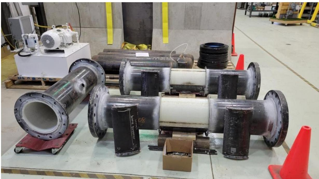
4. Full-scale tests for external loads and deformations associated as a minimum with vibrations, deflections, transverse ovalization, axial deformation, bonding/de-bonding at the coating/liner/pipe interface, internal pressure, and puncture
