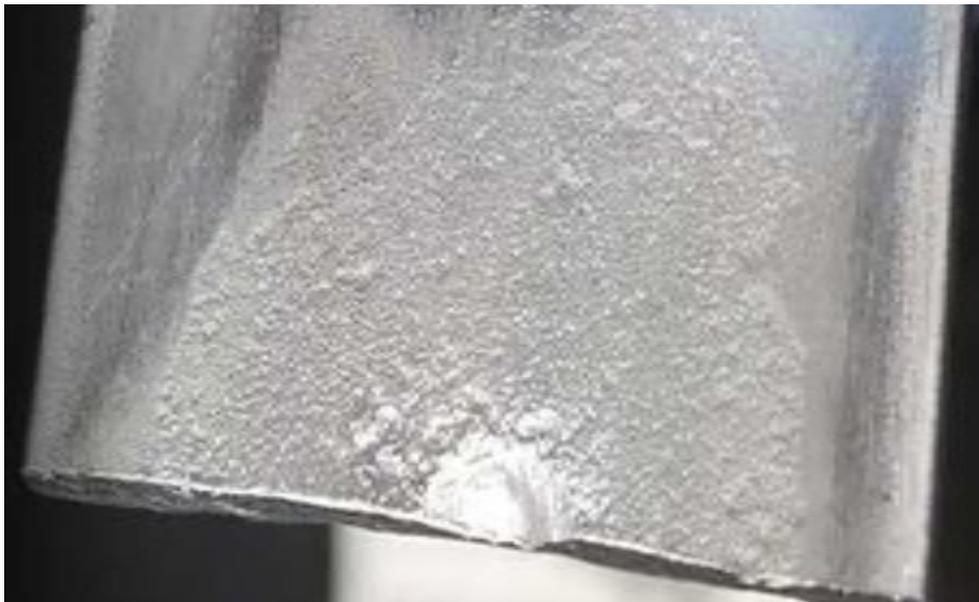
*Mercury damage to aluminum.*
