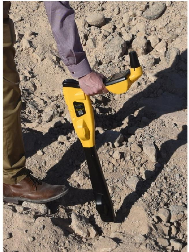
*A device for evaluation with a high-accuracy real-time kinematic GNSS receiver embedded in the locator itself. This type of receiver is preferable to a GNSS receiver embedded in the display/head of the locator, where it is difficult to have*
