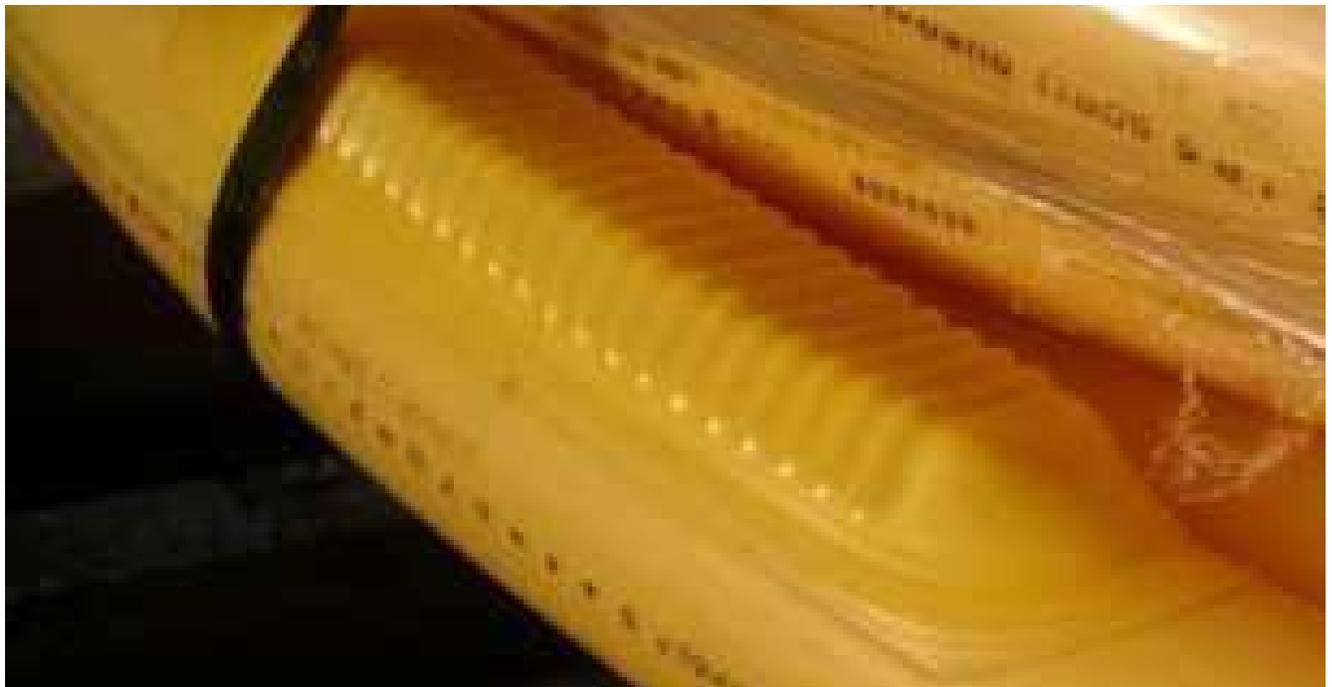
*PE pipe with locatable tags attached.*
