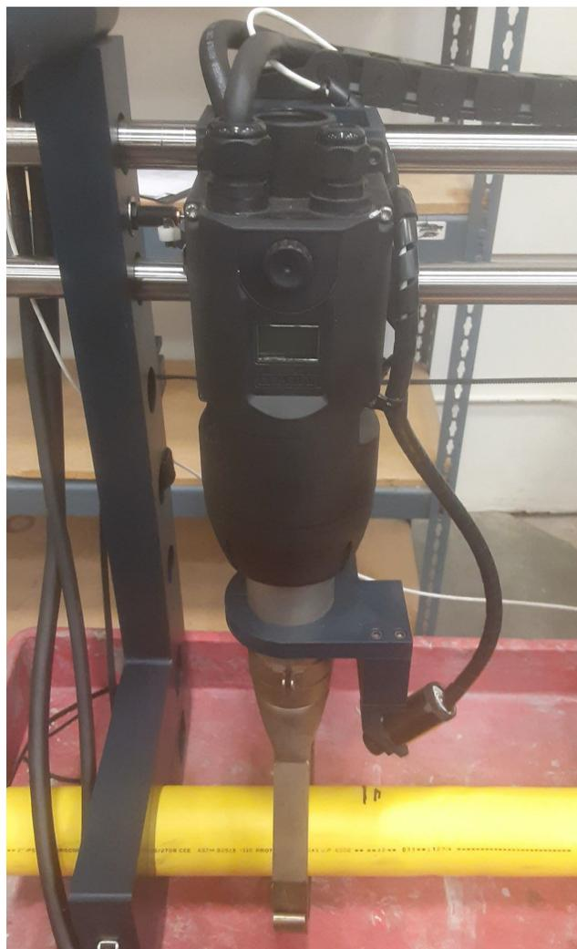
*PE pipe repair machine heating tool assembly.*
