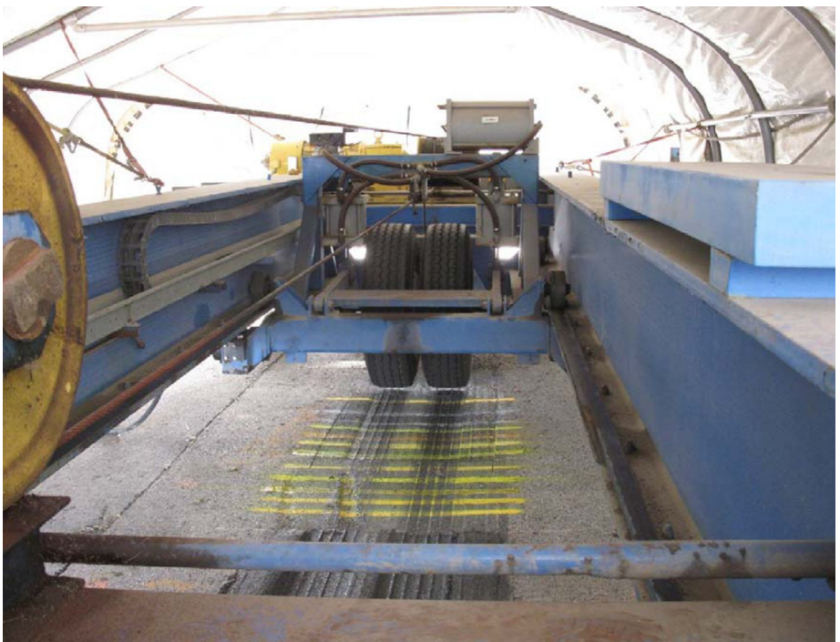
Paints were subjected to numerous evaluations through UV testing, water immersion, vehicular testing, and other examination techniques.
