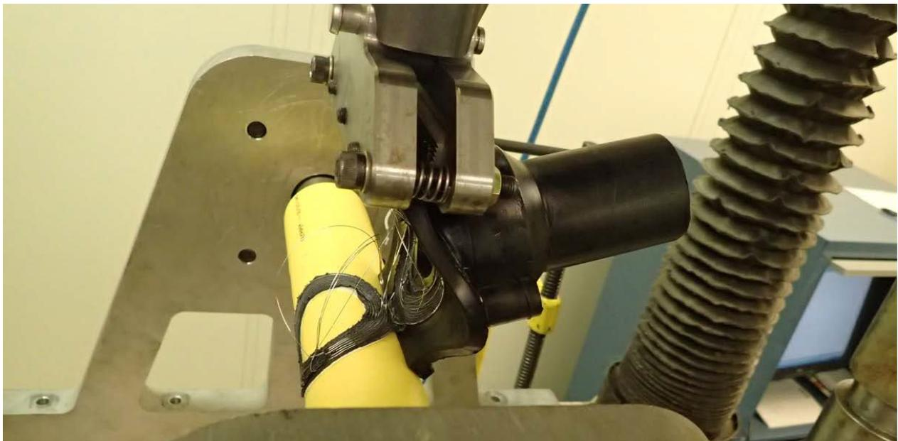
Example of saddle decohesion test.
