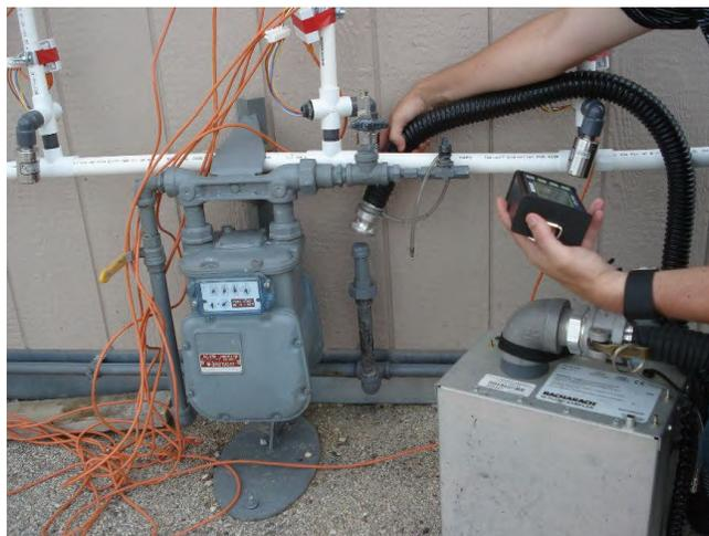
performed primarily to compare the leak plume image with the results of the gas sensors.
