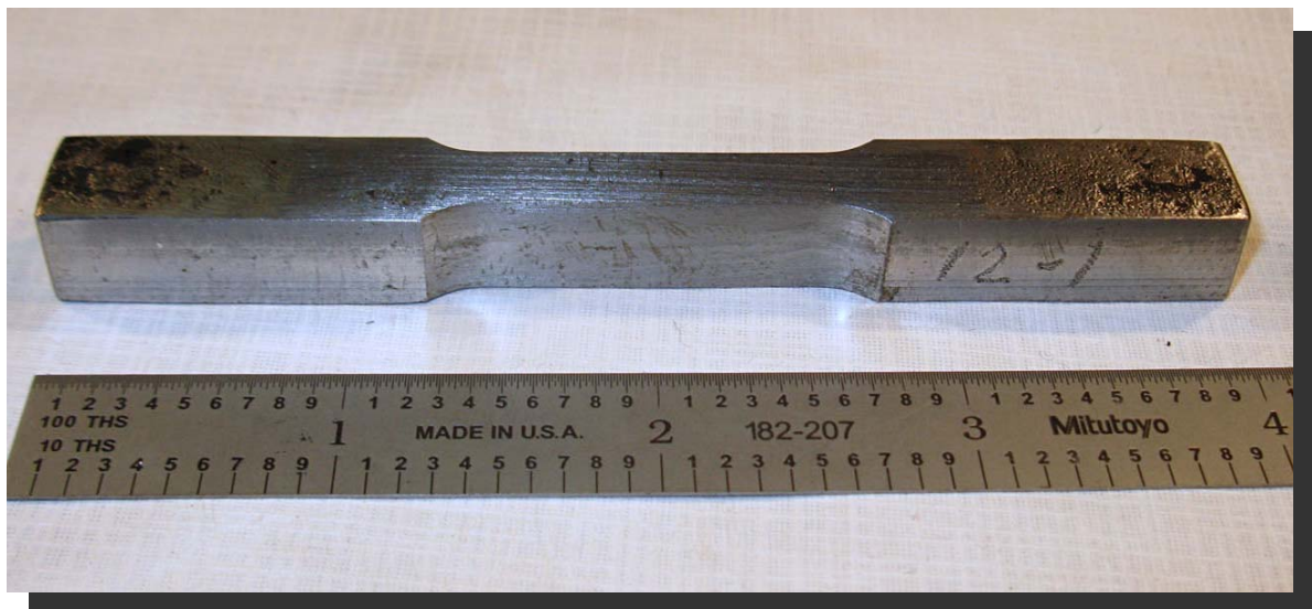
Research was conducted to determine if small pipe specimens can provide the same testing results as larger samples that are more costly to extract and test.
