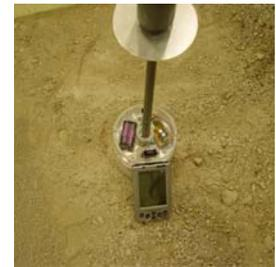
The DCP uses a five-pound drop-weight to drive a small cone into the soil, counting the number of drops required to penetrate the soil a fixed distance of 3-1/4 inches. The number of drops is determined by calibrating the device to the relative soil compaction of various soil types. Researchers report that the device proved to be a practical replacement for the nuclear density gauge by providing layer-by-layer compaction verification.
