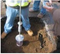
Throughout the natural gas industry, utilities use a variety of tools to measure soil compaction to ensure that adequate pavement restorations are provided following repairs or rehabilitations. In efforts to improve the overall effectiveness and lower the cost of pavement restorations, modifications were made on several soil-compaction measurement devices.
