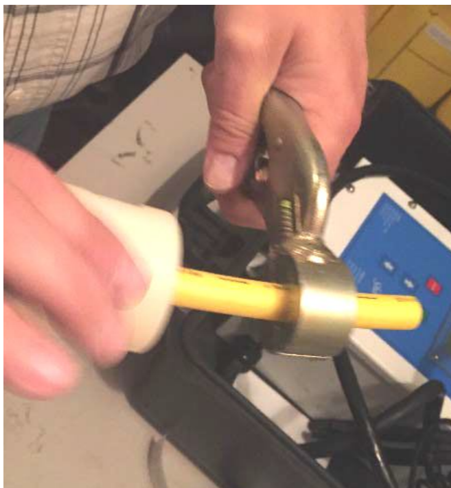
Testing of a pencil scraper on a 1/2-inch plastic tubing.
