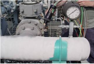
Researchers have investigated the use of thermal spray coatings (TSC) for long-term pipeline corrosion protection. Applicable in various pipeline environments, the technology is especially beneficial for use in critical locations and on pipelines that are difficult to access. Data developed through this project will advance TSC technology and provide pipeline operators with information to enhance the integrity of their systems.
